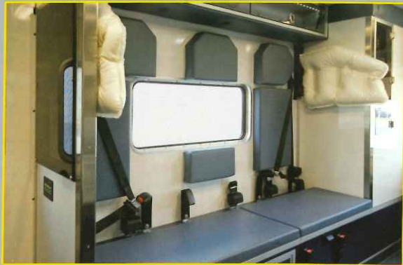
Two types of airbags are deployed in a side impact rollover collision: the Inflatable Head Curtain protects the attendant from the inhalation area cabinet and (optional) the attendant at each end of the bench seat. The Tubular Structure airbag is used with the attendant and the CPR seats for additional head protection.
