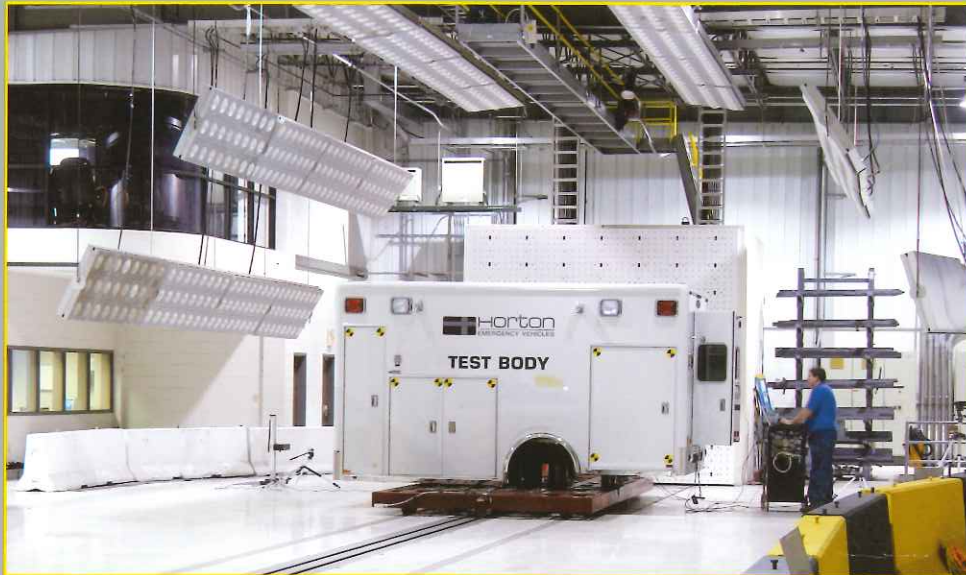
HOPS testing was conducted at the Center for Advanced Product Evaluation (CAPE ® ), a modern crash-test facility on the campus of IMMI. Above: a technician preps the sensors, high speed cameras and data collectors before a side impact test. Right: rollover impacts are created with this massive frame, the only one of it's kind in the world.
