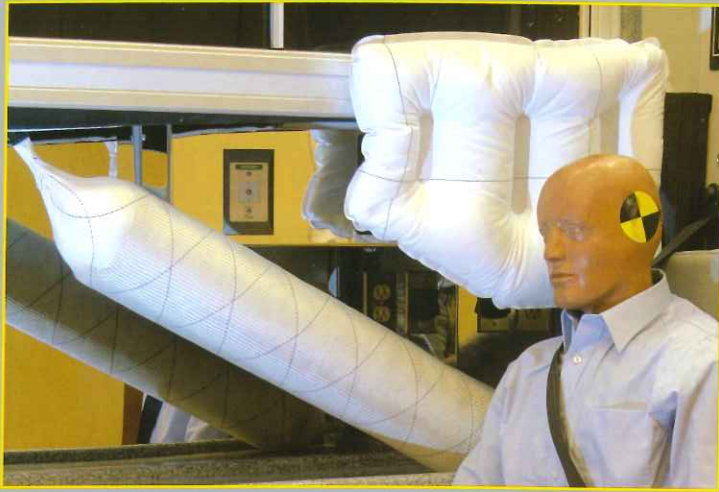
Two types of airbags are deployed in a side impact rollover collision: the Inflatable Head Curtain protects the attendant from the inhalation area cabinet and (optional) the attendant at each end of the bench seat. The Tubular Structure airbag is used with the attendant and the CPR seats for additional head protection.
