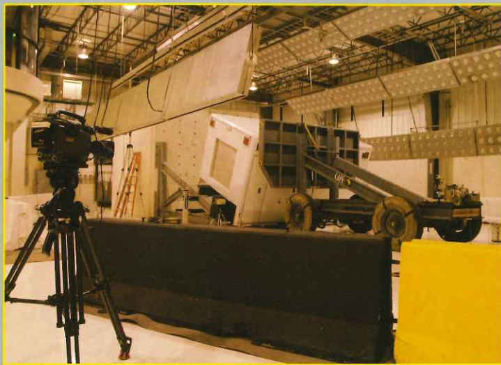
European and SAE standards dictate a series of tests to address survivable space around its occupants. Reasoning that if a cab occupant is entitled to certain crash protection, then certainly someone in an ambulance patient compartment should enjoy the same protection, Horton applied these same tests.
