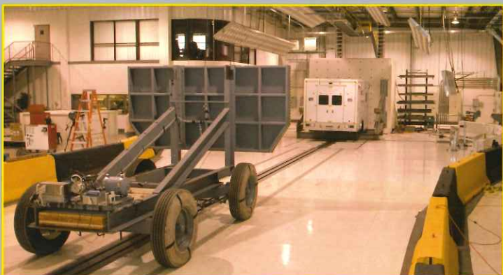
Far exceeding any structural requirements of the KKK specifications, this testing marked the first time in history such survivability testing was done on an ambulance body and clearly demonstrated the structural integrity of the Horton body. The tests were run with all cabinetry in place to demonstrate they would not detach and injure the occupants.
