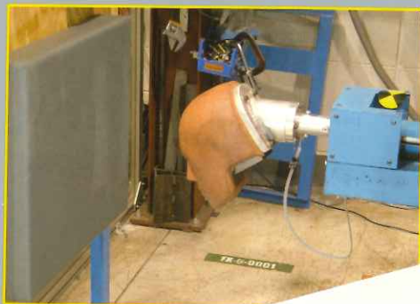
A head-strike cannon was used to test the HOPS cushion system.
