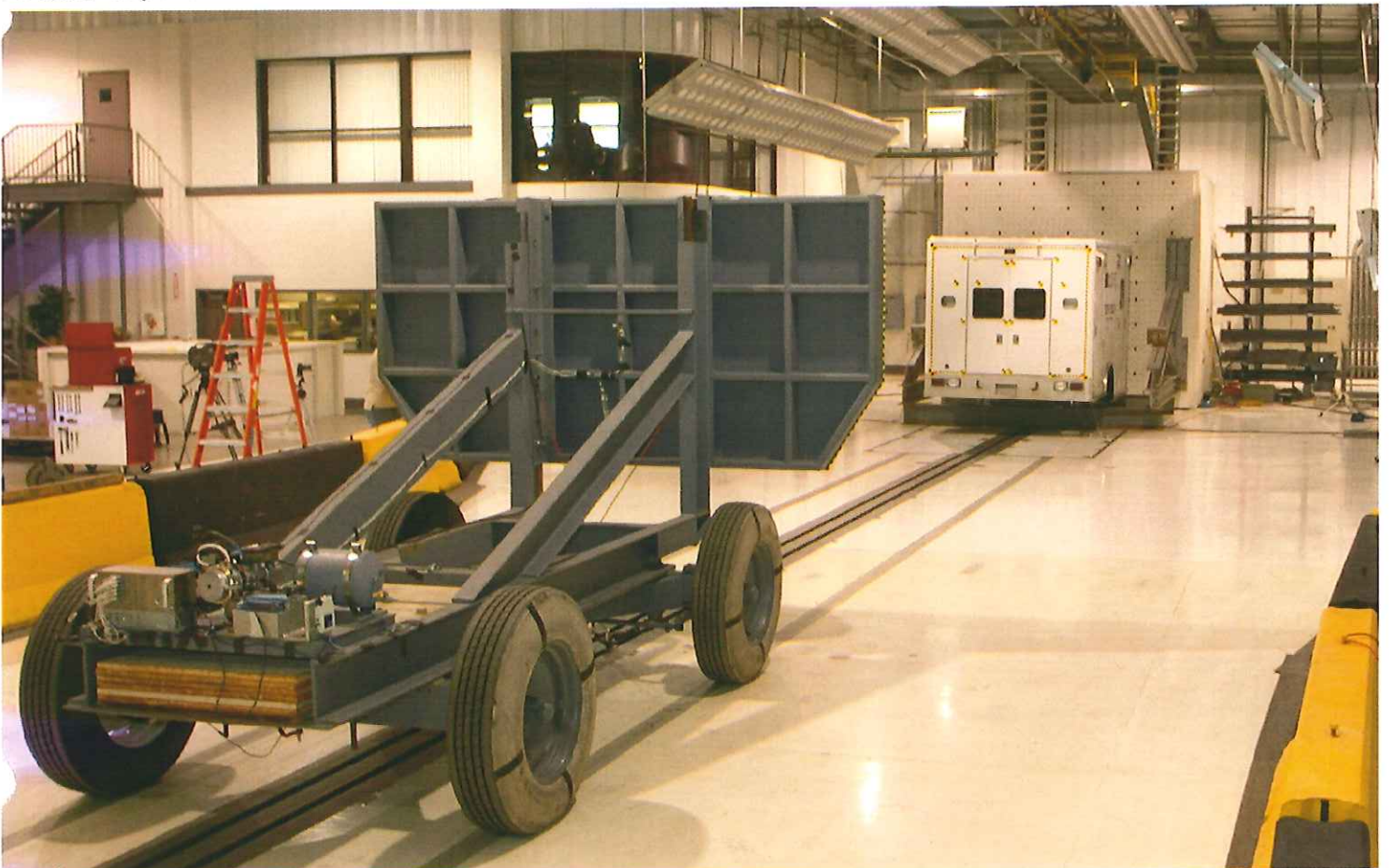
Rear Impact Test
