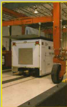
European and SAE standards dictate a series of tests to address survivable space around its occupants. Reasoning that if a cab occupant is entitled to certain crash protection, then certainly someone in an ambulance patient compartment should enjoy the same protection, Horton applied these same tests.
