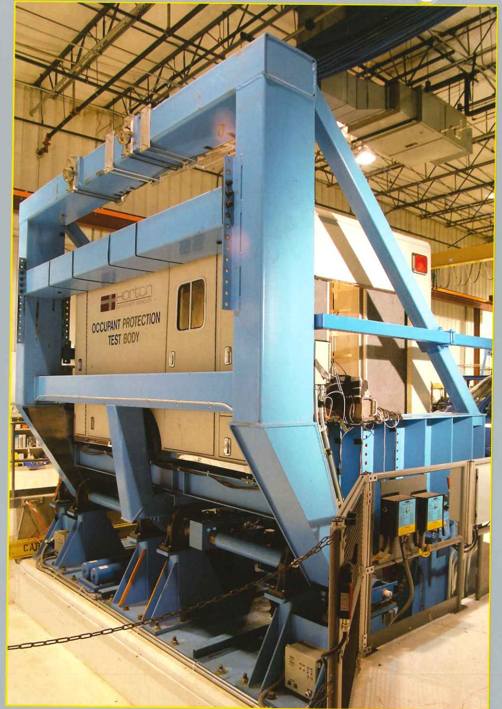
The dynamic rollover test machine enables test engineers to simulate a rollover event while recording significant test data from inside the vehicle. The Hybrid III test dummies are fully instrumented to check head strike impacts, G loads, neck loading and seat belt forces. Comparisons are made to evaluate base line data against data collected with new experimental systems and to ensure the efficacy of the solution. The Horton body was subjected to 14 rollover impacts and retained its structural integrity through it all.
